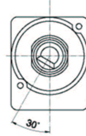
shaft shown in full C.C.W. position
